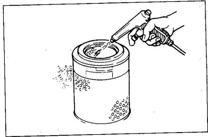
Figure 5. Dry Cleaning the Air Cleaner
