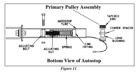
Clean all parts with a mild sovent such as WD-40 and be sure to dry all parts. Use a brush to insure the inside of the AutoStop tube is clean as well.
