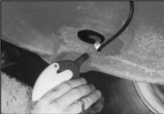
Leak test all air line connections. Repair or replace as needed. See page 7 to repair.
