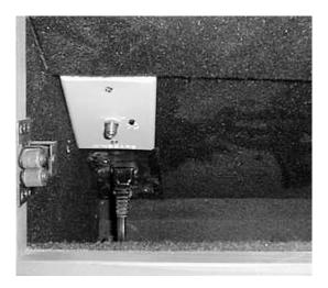
Turn **ON** the power boost. It is located in the front overhead cabinet. The boost draws 12 VDC power to amplify the antenna signal. A small switch in the overhead cabinetry in the front of the coach controls it. Since this does draw a small amount of house battery power, remember to turn it off when not in use.
