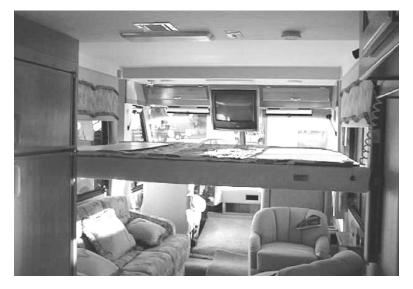
Your Trek is equipped with a space-saving ElectroMajic<sup>TM</sup> overhead bed. During the day, the bed is hidden in the ceiling of the coach. At night, it lowers down to make a comfortable bed. It is quick and easy to move while using 120 Volt power from the shore line connection, generator, or inverter.
